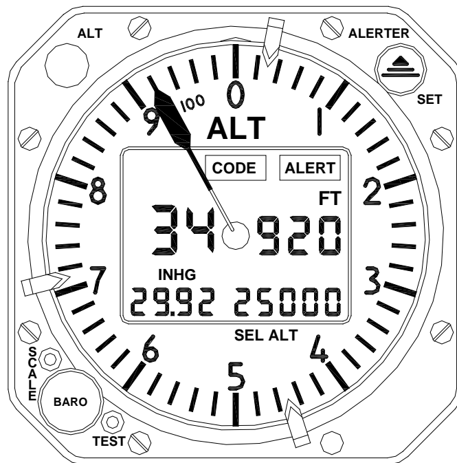
Figure 20: AD3X.(.) Baro Pot Output Version
