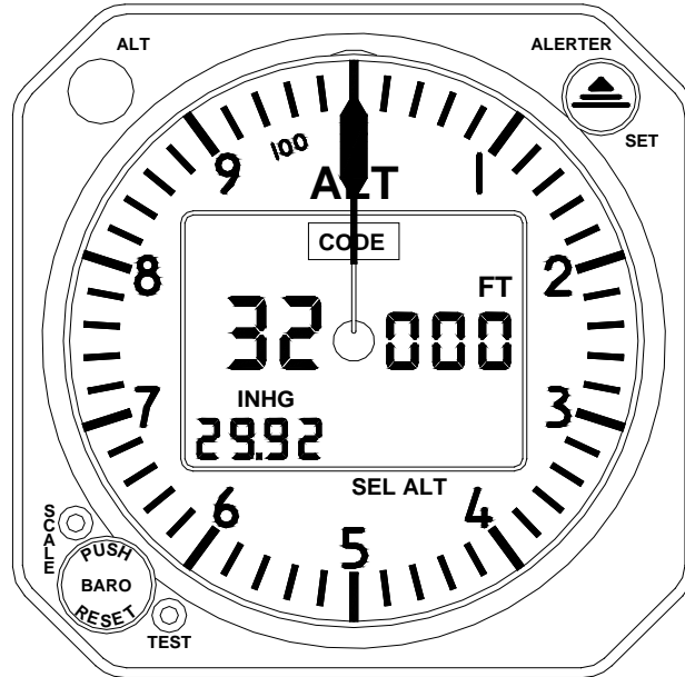
Figure 16: AD3X.(.) Indication of 'CODE' or Encoding Failure
