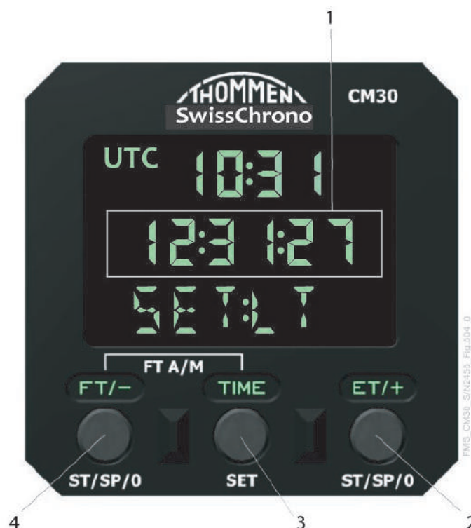
Figure 5 – Manually Setting the Local Time (LT)
