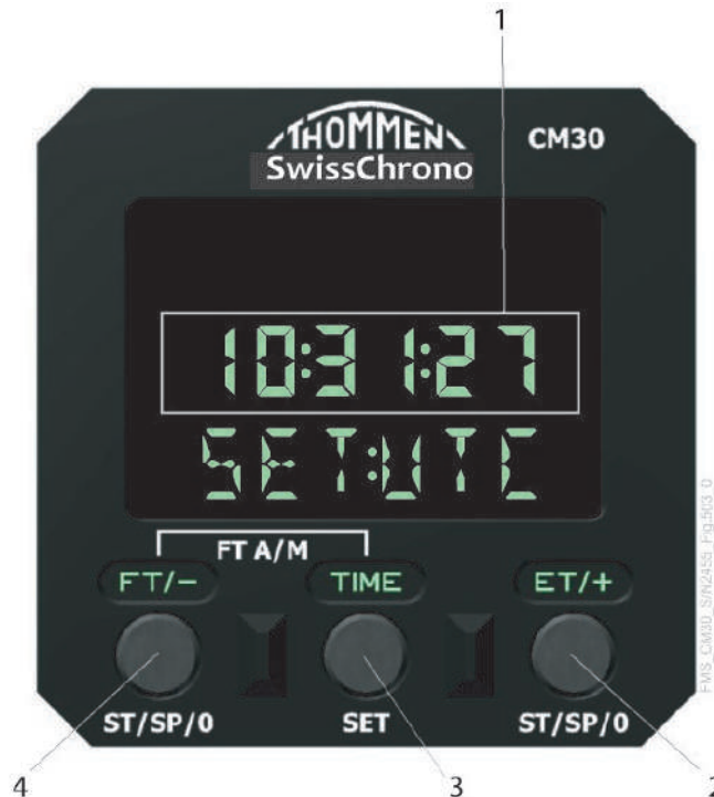
Figure 4 – Manually Setting the Universal Time Coordinated (UTC) Time
