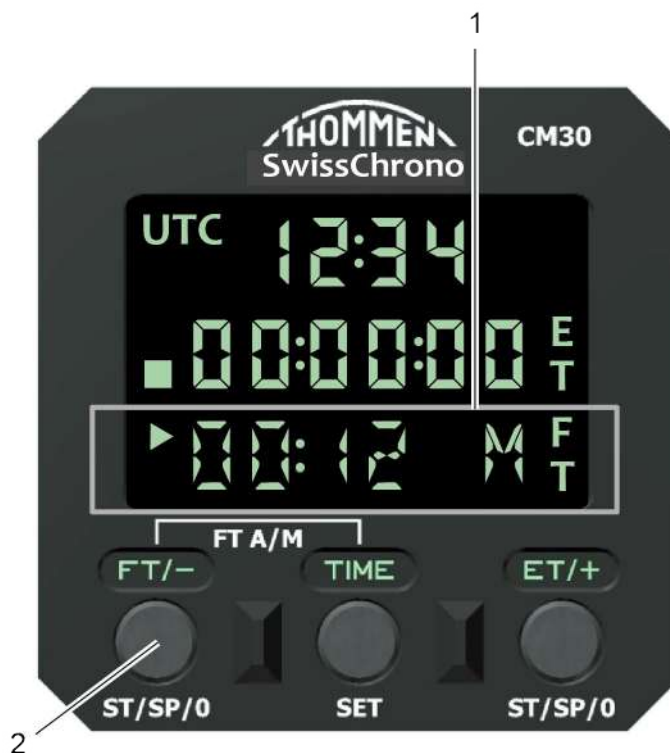
Figure 7 – Manually Start/Stop the Flight Timer (FT)
