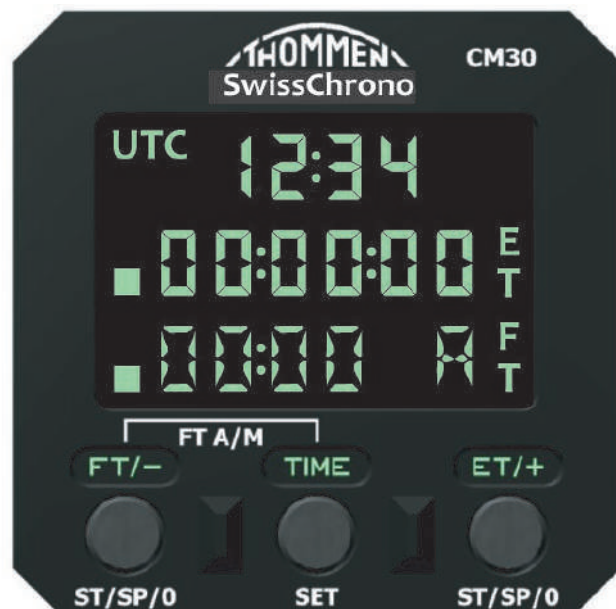
Figure 3 – After Five Second Start-up Built-In Test (SBIT)
