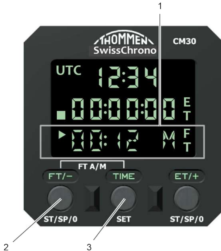
Figure 8 - Changing between Manual and Automatic Flight Timer (FT)
