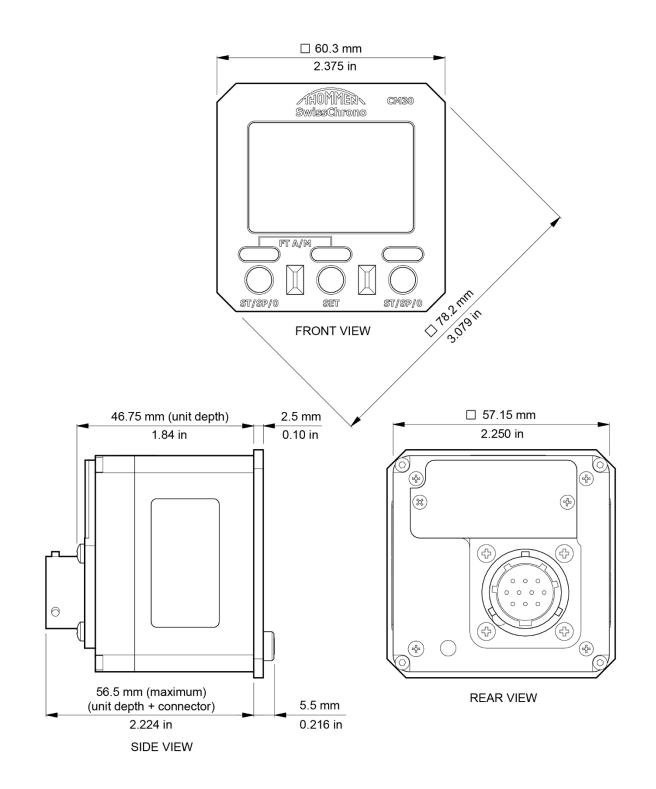
Figure 1 – CM30 Digital Chronometer – Physical Dimensions
