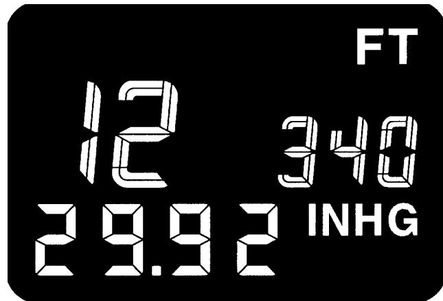
*Fig. 2-6 Display current altitude and baro setting*
