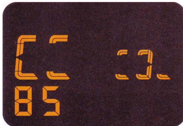
*Fig. 2-4 Display of battery charge / amber lighting (optional)*
